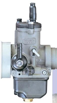
tor is equipped. To enrich we have to close the air screw (by closing the airflow) or open the mixture screw. To lean the mixture, one has to open the air screw or close the mixture screw.
