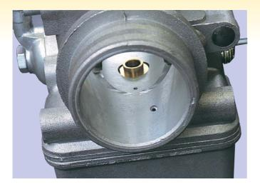
Below, with the throttle valve partially lifted, we can notice the arrangement of the progression port.
