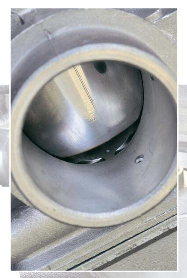
Above are two details of the supply ports of the idle and progression circuits, which can be seen slightly downstream of the main spray nozzle.
