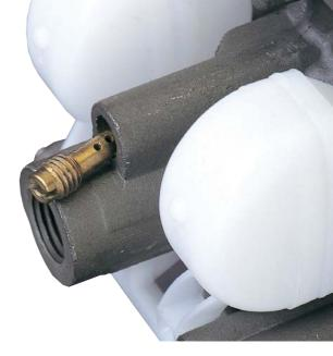
port. This progression port is placed upstream of the rear edge of the valve, just before the idle port (with respect to the direction of the airflow in the diffuser).
