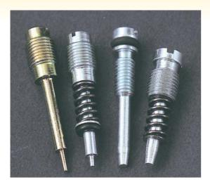
*On the left side we see a VHSC with the air adjustment screw near the aspiration mouth.*
